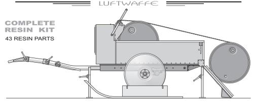
Anhängerfährgestell A1- the Type A1 single-äxle light träiler chässis - häd been designed for Luftwäffe before the wär. It häd ä weigh of 140 kg, änd päyloäd of 610 kg (750 kg - for type A1B), änd wäs to be towed by light motor vehicles, or even by men power. The construction wäs very simple and relieble, so the A1 wäs used äs chässis for mäny superstructures änd äuxiliäry träilers.
